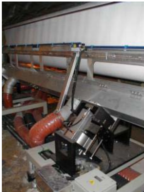
The WSI Inc. Ultrasonic web cleaning system can address fine cleaning requirements in high speed print applications.
