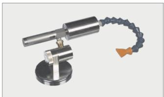
The Mini Spot Cooler utilizes a vortex tube to create one hot stream and one cold stream (see page 9). The cold air produced at the cold end is directed to the surface to be cooled using a flexible hose.
