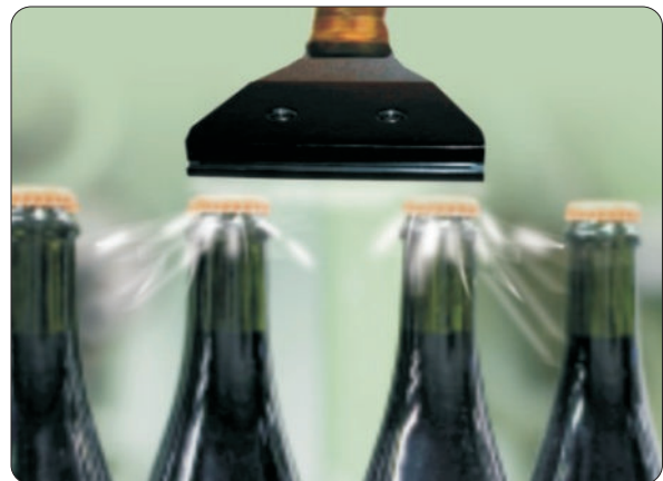
Air Edger™ Flat Jet with .008” gap setting blows water from under the caps on a bottling line moving at high speed
